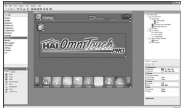
Use Leviton Automation Studio software to add particular hardware to the system or modify the appearance of the Touchscreen graphic interface.
