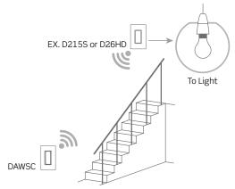
Add additional ON/OFF control at the base of a staircase
