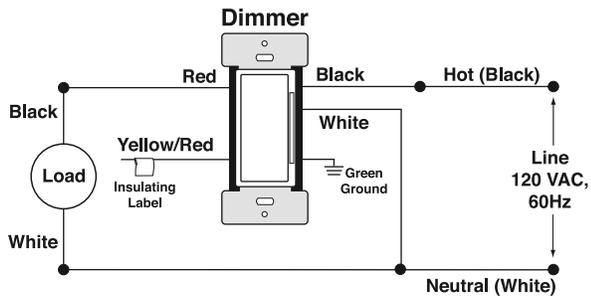
**THREE-WAY WIRING DIAGRAM**
