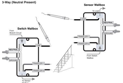
NOTE: Sensor must be installed in the location where the load wire is.
