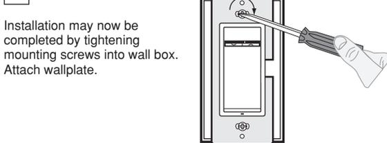
Installation may now be completed by tightening mounting screws into wall box. Attach wallplate.
