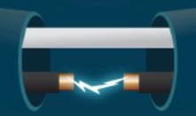
**Series Arc:** Arc along the same conductor or at connections.
