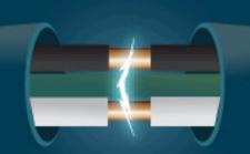
Parallel Arc: Arc between the hot and neutral conductor or between the hot and ground conductor.
