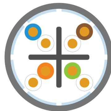
SEZIONE TRASVERSALE CAVO U/UTP CON NASTRO LAMINATO DISCONTINUO
