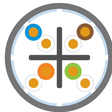
DISCONTINUOUS FOIL TAPE U/UTP CABLE CROSS SECTION
