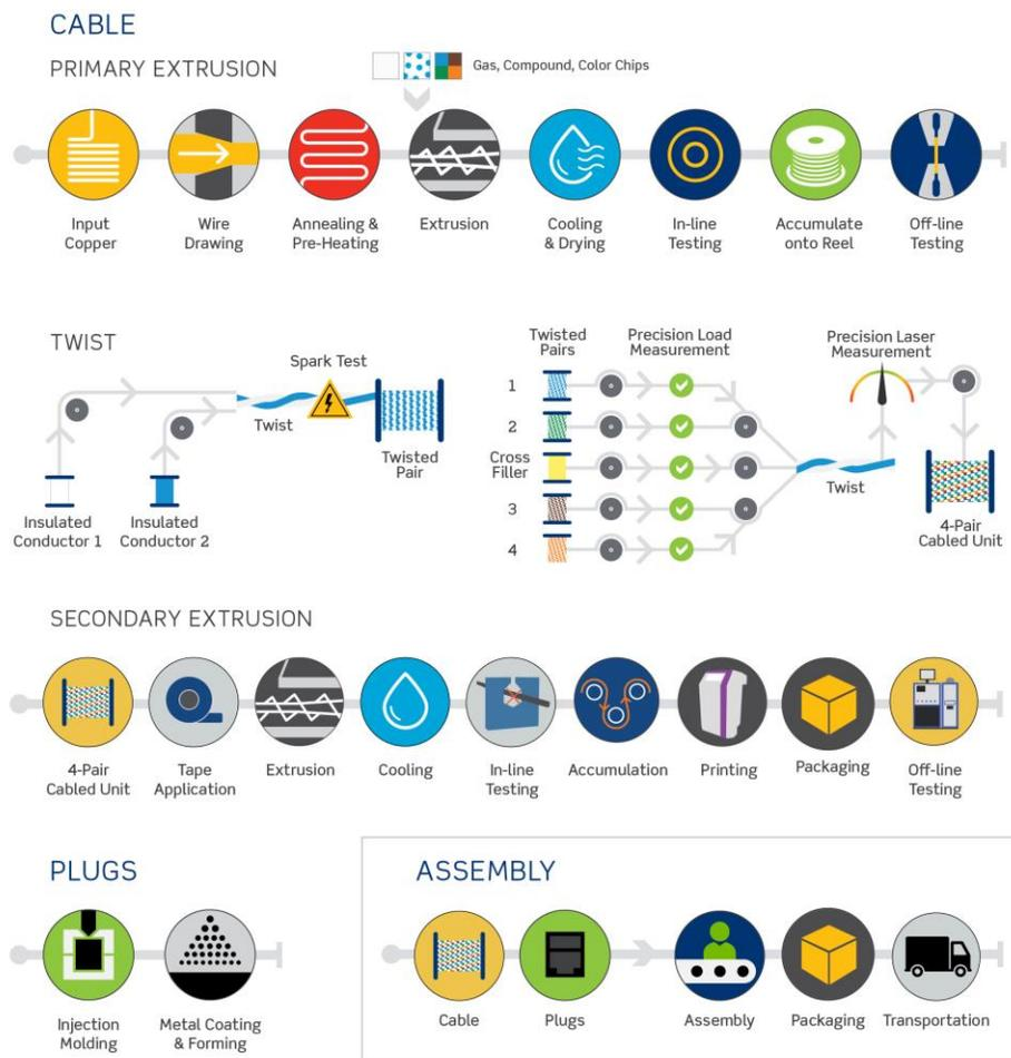
Figure 1: Patch Cord and Consolidation Cord Manufacturing Process
