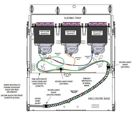
When used in an HDX Patch Panel the modules install from the front side only. Cabling is dressed on a rear cable manager, passed through to the front side of the panel and splice modules are terminated.
