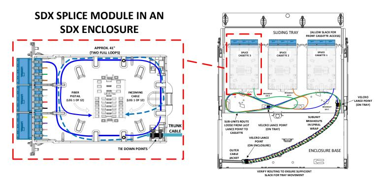
\*NOTE: SDX Splice Modules are installed from the front side of an enclosure or panel only. SDX sliding trays can be removed rearward to perform terminations.
