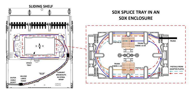
\*NOTE: SDX Splice Trays are accessible from the rear of a fixed or sliding tray enclosure. Sliding trays are removable from the front or rear.
