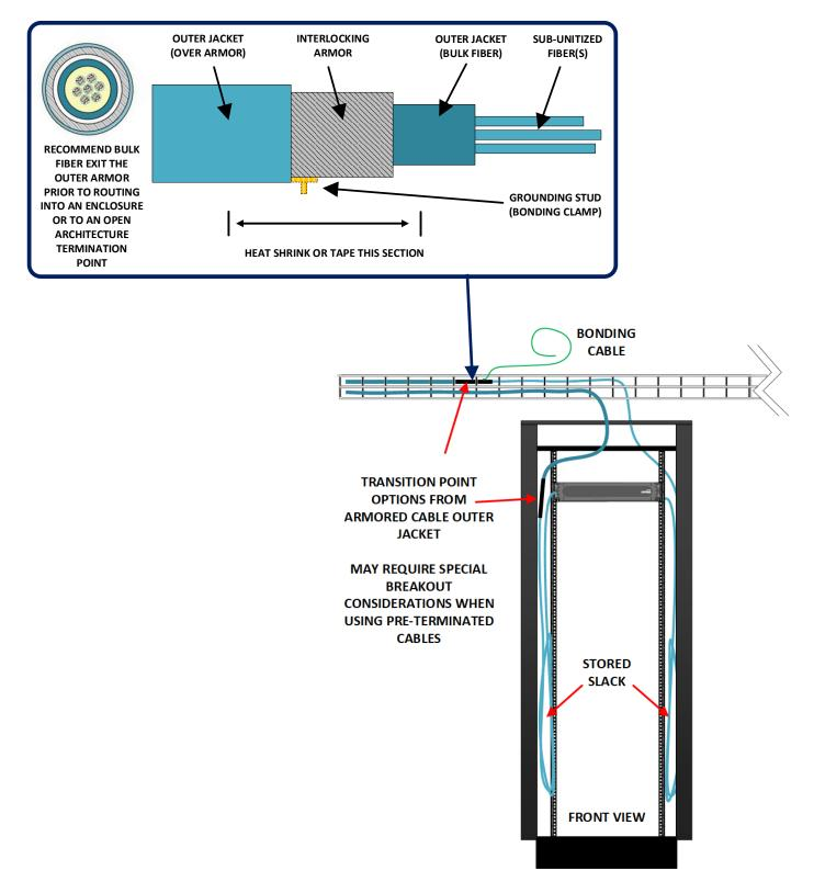
The following are examples of recommended routing methods for SDX splice trays and HDX splice modules.
