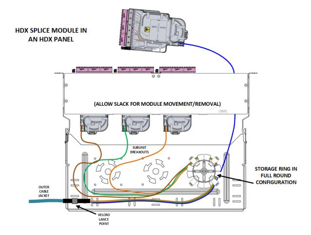
When using an HDX patch deck, the modules are loaded from the front. The individual trays also slide rearward to perform terminations.
