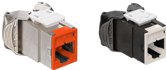
QUICKPORT ATLAS-X1 shielded and unshielded jacks. Category 6A jacks (part numbers 6ASJK-xx6 and 6AUJK-xx6) shown. ATLAS-X1 jacks are also available in Category 6 (part numbers 61SJK-xx6 and 61UJK-xx6).
