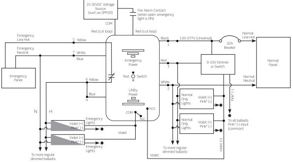
NOTE: Red wires are polarity independent; normal only lights are optional. \*Depending on date of manufacture, pink wires may be gray.
