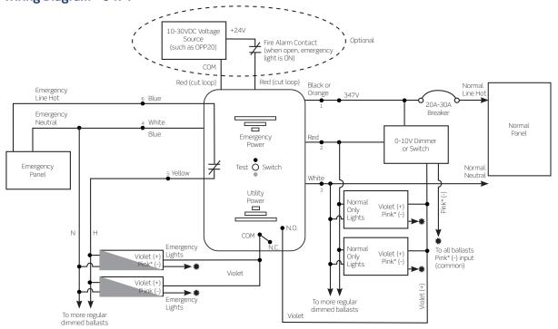
NOTE: Red wires are polarity independent.
