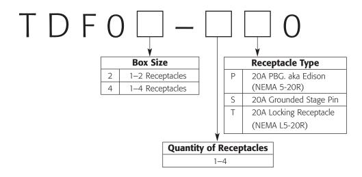
Order example: TDF3-4TD, indicates a 1-3 receptacle size box with 4 locking plug receptacles and 1 DMX out. Circuit Numbering: Receptacles will be labeled as per documentation at time of order. In cases where circuit numbers are not known, field circuit labeling kits can be provided.
