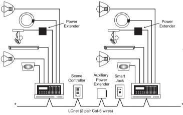
\*NOTE: First and last nodes (devices) on LCnet must be terminated.
