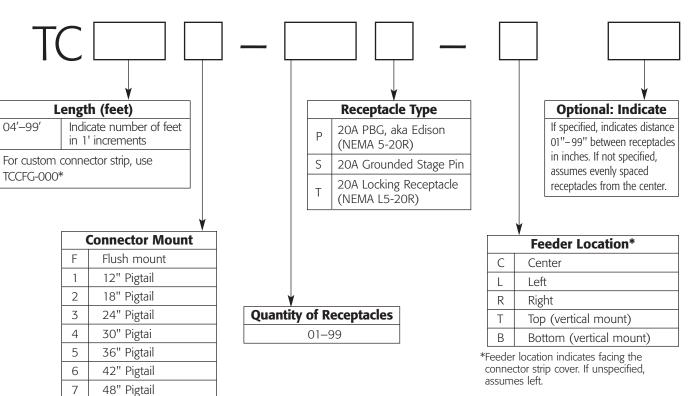
Order example 1: TC45F – 24S, indicates a 45' long connector strip with 24 evenly spaced flush mounted stage pin receptacles and a feeder location\* on stage left end of the connector strip.
