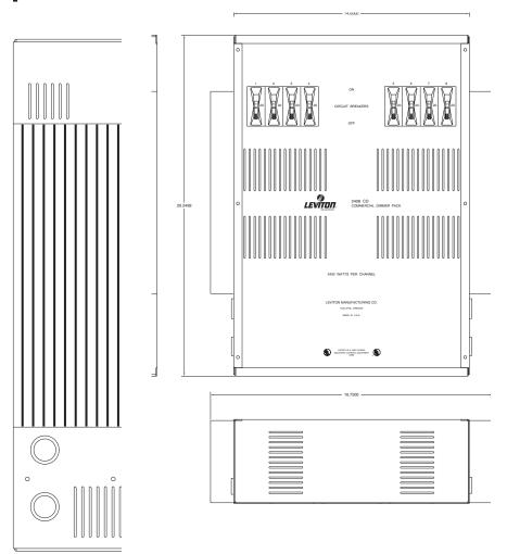
These UL listed commercial dimmer packs feature input ports for all the communication protocols you'll need, including NSi's Micro-Plex, DMX512, NSI Luma-Net® and o-10V analog. The 2408 also features epoxy encased toroidal filters, which minimize noise and have a rise time of 400 microseconds. Combine with Luma-Net control stations or any Leviton-NSI control console for a totally integrated lighting system.
