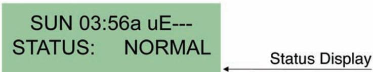
When the system is operating normally, the top line of the LCD display shows the day, time, locked/unlocked status of the panel, and the status of the event scheduler. The second line shows the status of the panel: Normal, Bypass ON, Bypass OFF, or Emergency.
