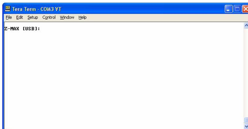
Since you will be replacing the operating system of the control board, you must jump out of the main operating system that is managing the communications and into a boot section of code that will perform the file transfer.
