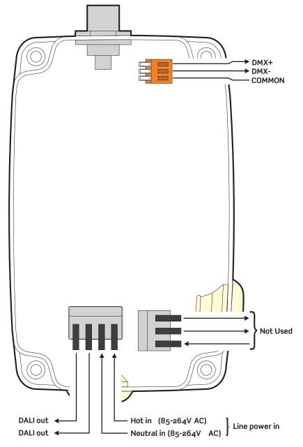
85-264VAC power input/output Warning! To avoid death, injury or property damage, Disconnect line power before connecting, disconnecting, or whenever opening the enclosure.
