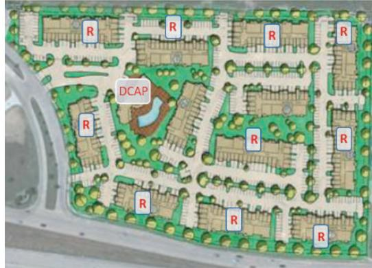
**2. Mid-Rise:** In this type of structure, repeaters are usually placed in service rooms and closets found throughout the property. These closets should be locked/secured and have power available. A thorough review of site drawings will help the planner to understand what locations are available and if alternative locations are required. It is best to avoid locations that do not already have power available.
