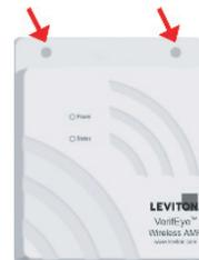
1. Select a location to mount the Repeater. Two mounting holes in the top of the cover may be used to attach to a surface.
