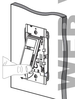
b. With the front faceplate of the sensor removed, push both buttons on front of sensor simultaneously for 10-15 seconds (note: after 5 seconds, a light will blink BLUE and then alternate between BLUE and RED) and release when the Locator Light is blinking GREEN.
