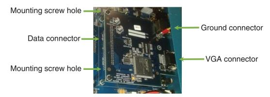
3. In sert VGA connector through hole in rear panel. 4. Insert data connector in socket (align properly). 5. Install power and ground connectors. 6. Install all mounting screws.
