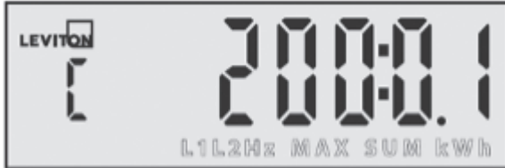
CT Amperage Startup Screen, No Error Conditions
