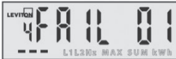
Error Screen Showing a Failure code, Factory Service Required
