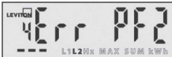
Error Screen Showing a Power Factor Installation Error on Line 2
