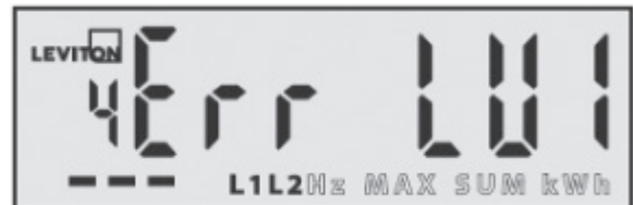
Error Screen Showing a Low Voltage Installation Error on Lines 1 and 2
