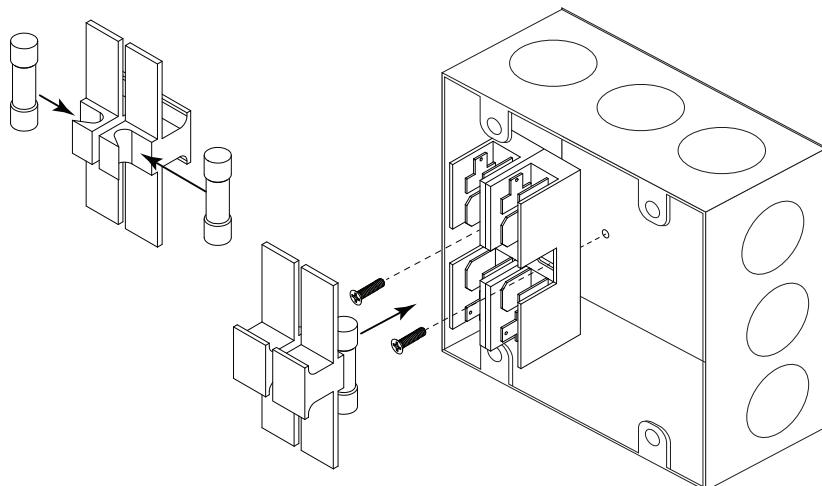
**2a. Wiring example 1** - The fuse is installed on the line side of the dimming control. Under this method, a single ECD00-FUS may feed multiple ECD00-D0Ws, provided that their total load does not exceed 16A and they share the same normal and emergency breakers.
