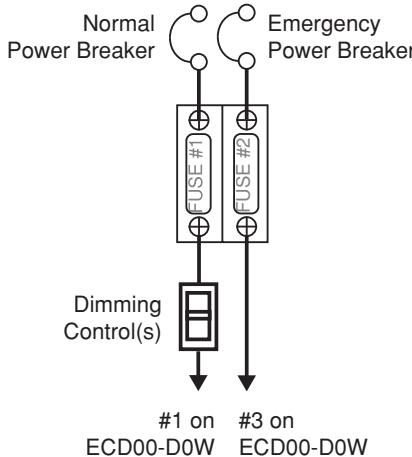
**2b. Wiring example 2** - The fuse is installed on the load side of the dimming control. Under this method, an ECD00-FUS is needed for each ECD00-D0W.
