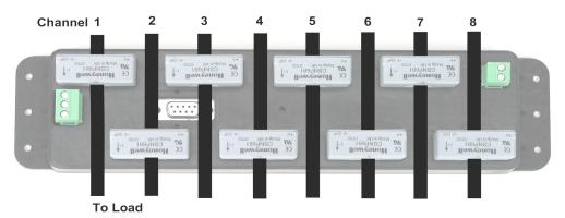
This illustration shows the 8 load wires passing through the individual hall effect sensors. The channel number for each load wire is shown at the top.
