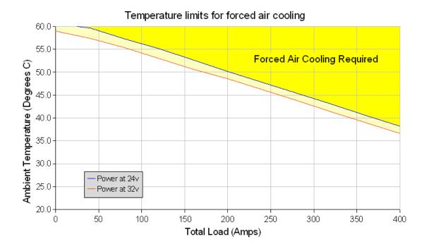
When using the chart above, the total current being monitored on all 8 channels should be used averaged over a 1 minute period. The chart assumes long term current levels at a steady state. Infrequent peaks lasting less than 30 seconds (such as inrush current) should not be used for this calculation.
