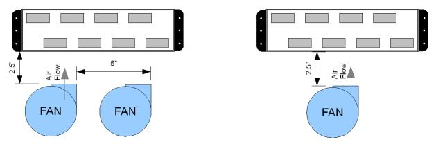
The examples show use of a single fan and two fans. While airflow from a single fan is acceptable, two fans provides some redundancy in case of mechanical failure. The fan should be capable of at least 10cfm. A thermostatic switch can also be used to turn on the fan above specific temperatures.
