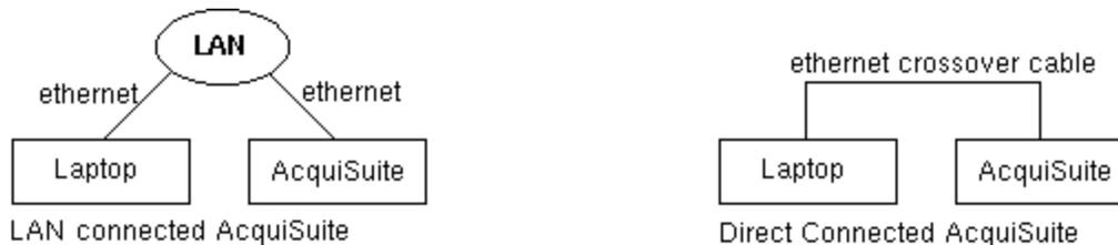
The remainder of this section will assume the installer has brought a laptop to the site, and will connect the laptop to the building LAN, or directly to the AcquiLite. Attach the laptop to the AcquiLite or LAN as shown in figure 6, Ethernet hookup.
