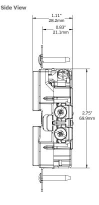
\*Self-grounding when installed in a properly grounded metallic box
