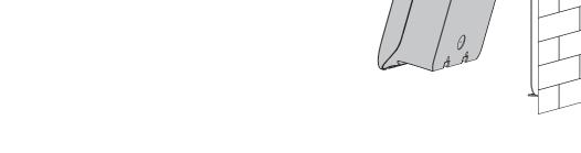
8. Slide the charger into place and align the screw holes at the bottom. Secure the charger using the previous removed screws.
