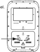
4. Remove the waterproof plug from the cabel inlet.
