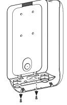
4. Lift the mounting bracket away from the charger to remove the mounting bracket.
