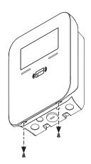
3. Remove the Wiring Access Panel. Use a flat-blade screwdriver to unlock the latches and remove the panel.
