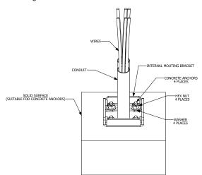
Install pedestal over internal mounting bracket using four (4) 1/4 in.-20 x 7/16 in. hex drive flat head screws.
