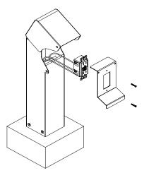
**9.** Place the wired device mounting plate into the pedestal by following steps 1-3, as shown in the images below.
