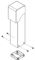
2. Use the supplied internal mounting bracket as a template, or use the dimensions shown in the diagram, and drill four mounting holes.
