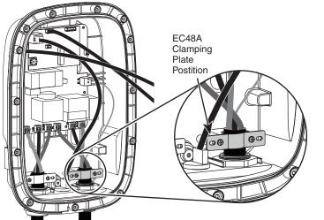
Install front cover to back cover and secure with 13 screws. Torque screws to 8.5 - 10.5 in-lb.
