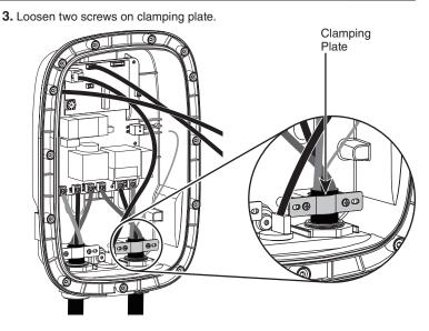
4. Loosen gland cap and remove cord.
