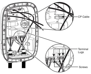
Tighten two screws securing clamping plate. Torque screws to 8.5 - 10.5 in-lb. NOTE: When installing EC32A 32 Amp replacement cord, concave side faces front cover.
