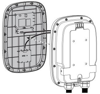
2. Remove three screws and cord terminal lugs from circuit board. Unplug CP cable.
