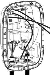
Plug CP cable into circuit board. Install cord terminal lugs to circuit board with three screws. Torque screws to 8.5 - 10.5 in-lb.
