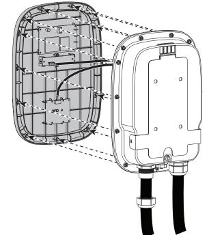
5. Tighten gland cap to seal. Torque gland cap to 8.5 - 10.5 in-lb.
