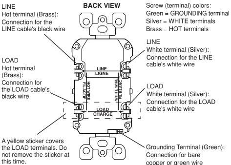
(a) Detach one cable's white wire and hot wires from the receptacle and cap each one separately with a wire connector. Make sure that they are from the same
