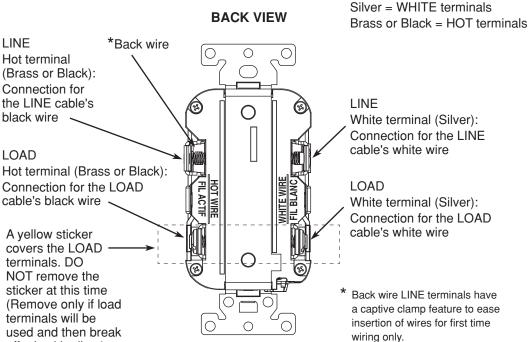
(a) Detach one cable's white wire and hot wires from the receptacle and cap each one separately with a wire connector. Make sure that they are from the
