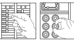
Next, plug in and turn ON the lamp or radio at the receptacle's other outlet to make sure the power is OFF at both outlets. If the power is not OFF, stop work and call an electrician to complete the installation.
