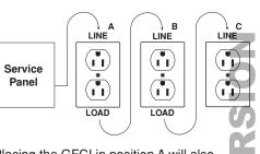
Placing the GFCI in position A will also provide protection to "load side" receptacles B and C. On the other hand, placing the GFCI in position C will not provide protection to receptacles A or B. Remember that receptacles A, B, and C can be in different rooms.
