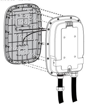
5. Tighten gland cap to seal.
