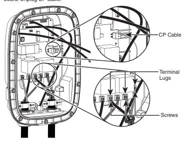
3. Loosen two screws on clamping plate.
