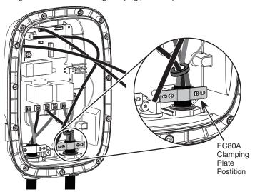
Install front cover to back cover and secure with 13 screws. Torque screws to 8.5 - 10.5 in-lb.
