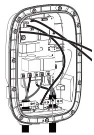
Plug CP cable into circuit board. Re-position the magnetic ring on the cable to be secured at terminal L1. Install cord terminal lugs to circuit board with three screws. Torque screws to 8.5 - 10.5 in-lb.
