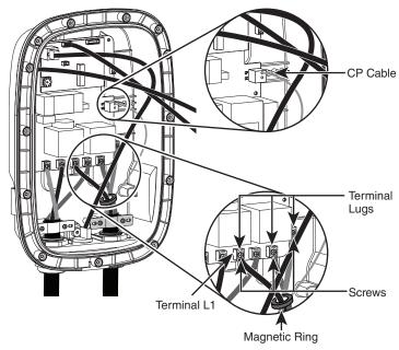
3. Tighten two screws securing clamping plate. Torque screws to 8.5 - 10.5 in-lb.
