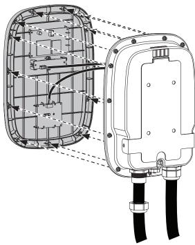
**5.** Tighten gland cap to seal. Torque gland cap to 8.5 - 10.5 in-lb.
