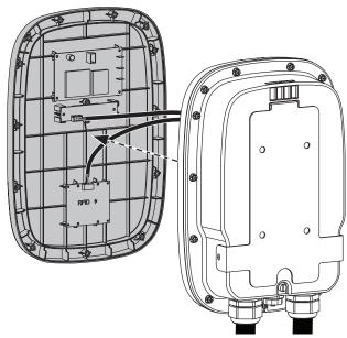
Remove three screws and cord terminal lugs from circuit board. Unplug CP cable.
