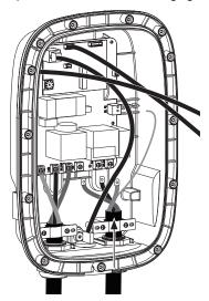
2. Plug CP cable into circuit board. Install cord terminal lugs to circuit board with three screws. Torque screws to 8.5 - 10.5 in-lb.
