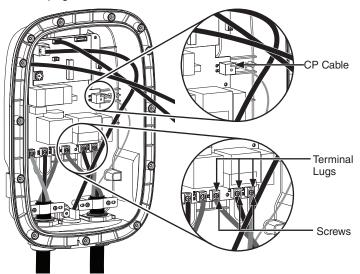
3. Loosen two screws on clamping plate.
