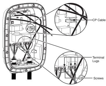
3. Tighten two screws securing clamping plate. Torque screws to 8.5 - 10.5 in-lb.
