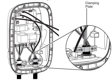
4. Loosen gland cap and remove cord.
