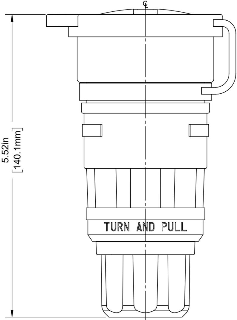
WETGUARD CONNECTOR SHOWN WITH CLOSURE COVER ASSEMBLED
