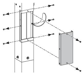
2. On both sides of the pedestal, remove the two square plates with the opening and the M5 x 14mm screws and set them aside.
