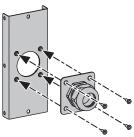
6. Install the improved wiring window in the same location where the holeless wiring window was using the eight M5 x 12mm screws (step 1) on front of the pedestal.
