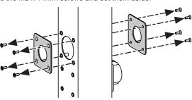
3. Replace the two plates with the holeless metal cover using the previously removed M5 x 14mm screws, or the screws provided in the kit.
