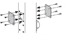
4. Assemble the connector and square plate with 1.5/8 in. (4.13 cm.) opening and matching nut.
