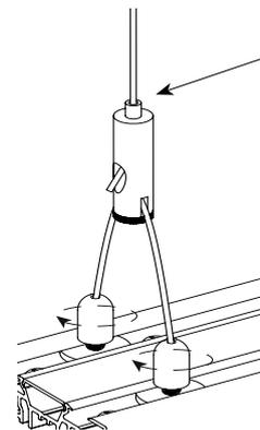
To adjust the cable length to level the luminaire or remove/reverse the direction of the cable the locking mechanism can be disengaged by pressing the nipple downwards as the cable is pulled. The cable can be trimmed if required.
