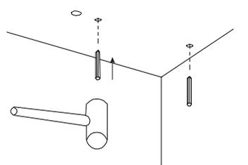
Drill suitable mounting holes in the ceiling for wall plugs (A) and insert.
