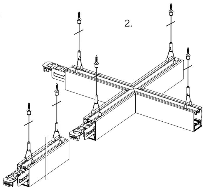
When installing Line of Light sections using the suspension kit, each section joint must be supported with a suspension wire to ensure that all joints are fully supported.
