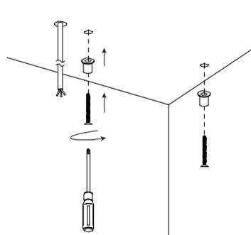
Screw the mounting cable cap (B & C) into ceiling.
