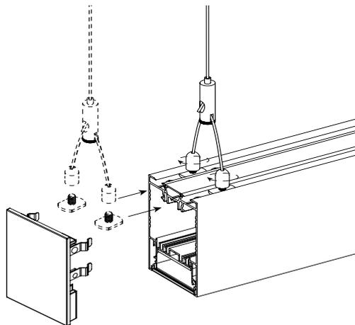
Remove end cap and slide captive screws (E) into the body channel as a above illustration and fit threaded caps until tightened, then refit the end cap.
