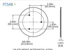
\* PLATE HEIGHT AFTER INSTALLATION IS APPROXIMATELY .20 INCHES [5.1mm]
