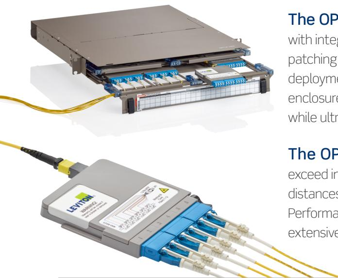
**The OPT-X HDX patching platform** improves network manageability with integrated cable management and port labeling in both closed- and open-patching options. OPT-X HDX Adapter Plates and Cassettes can accelerate deployment and MACs through easy one-hand installation and removal. HDX enclosures and panels offer manageable density at 96 fibers per RU (using LC), while ultra-high-density UHDX enclosures support up to 144 fibers per RU.
