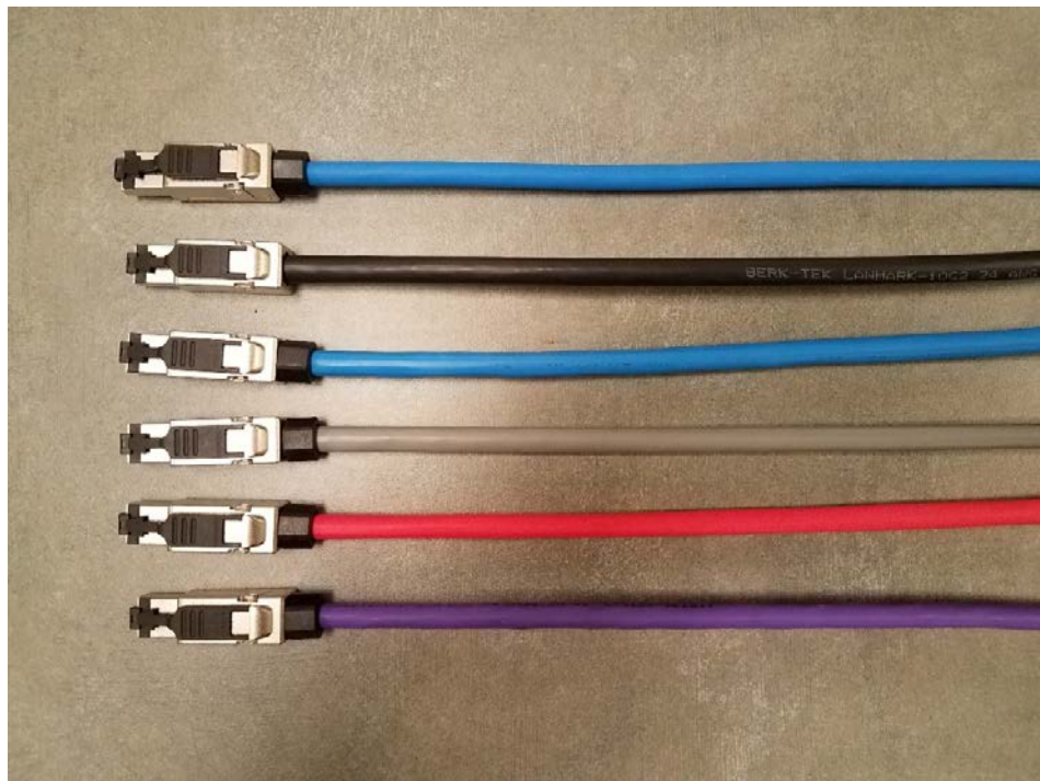
Leviton Category 6A Tool-free Universal Plug shown terminated on various Berk-Tek Category 6A Shielded and Unshielded (UTP) cables. Where cable jacket is slightly too large (over 0.300 inch OD) the rear nut assembly may be omitted (as shown on the black LANmark 10G2 CMR above) with no loss of termination integrity. (10G2 CMR has nominal OD of 0.320 inches).
